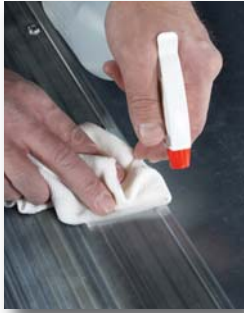
5 Simply clean with a solution of water and isopropyl alcohol and wipe dry.
